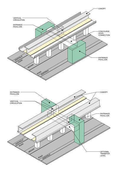
Figure 6-7: Elevated LRT Station above median - side platform
