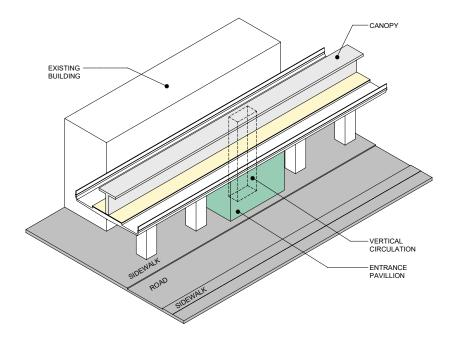
Figure 6-8: Elevated Station above sidewalk - centre island platform
