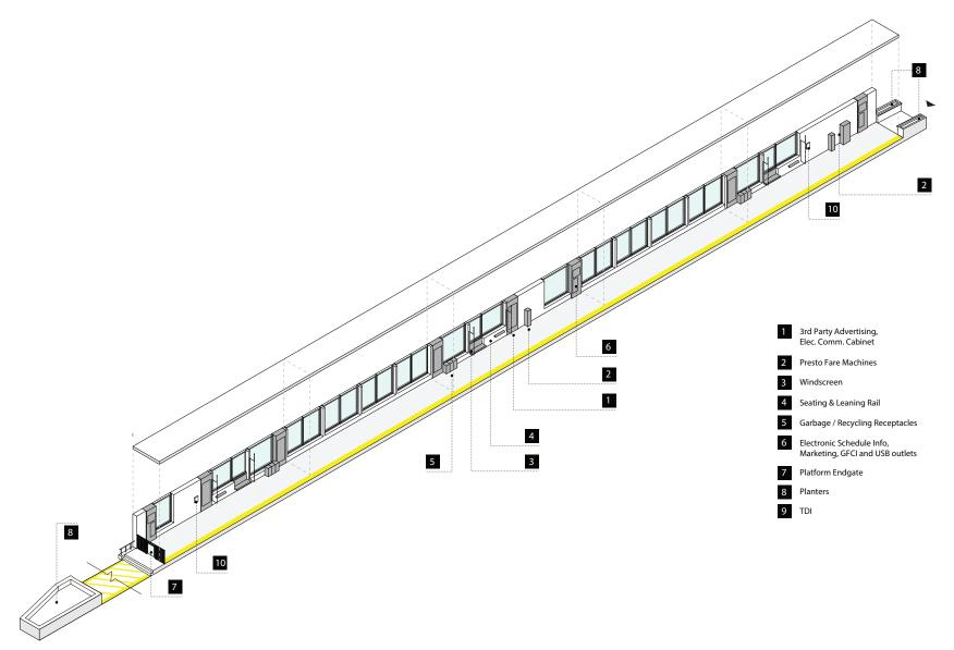
Figure 5-19: Shelter at median, Side Platform
