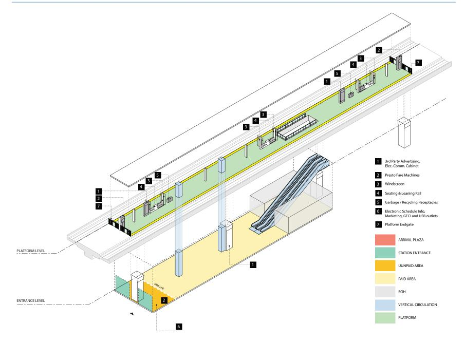
Figure 6-3: Elevated Station (axonometric projection)
