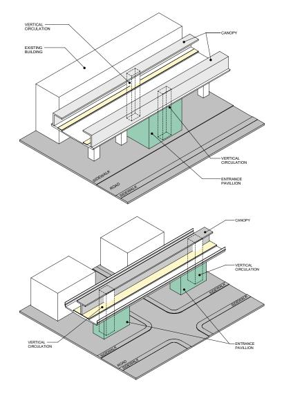
Figure 6-9: Elevated platform above sidewalk - side platform
