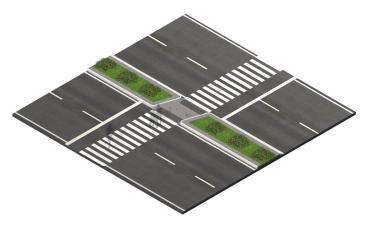
Figure 4-26: Median Refuge with offset cross-walk
