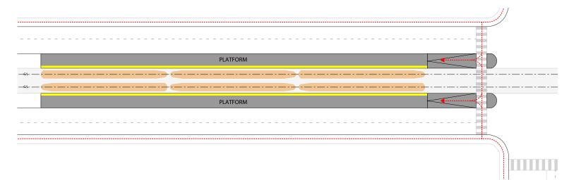
Figure 5-13: Horizontal Access - Centre Island Platform
