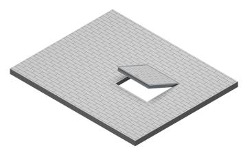
Figure 5-22: Access hatch
