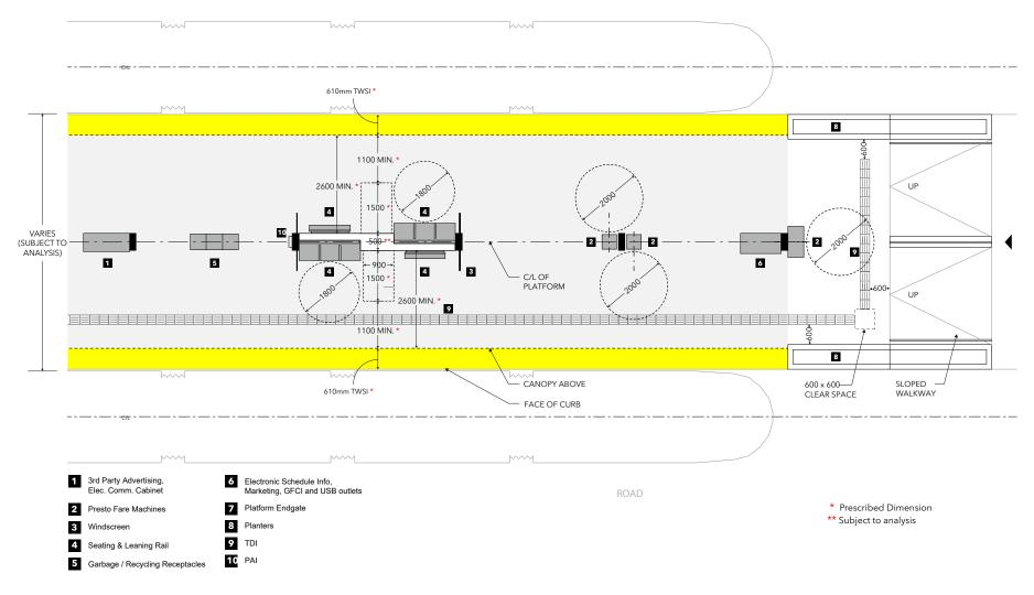
Figure 5-11: Enlarged plan of a typical centre island platform
