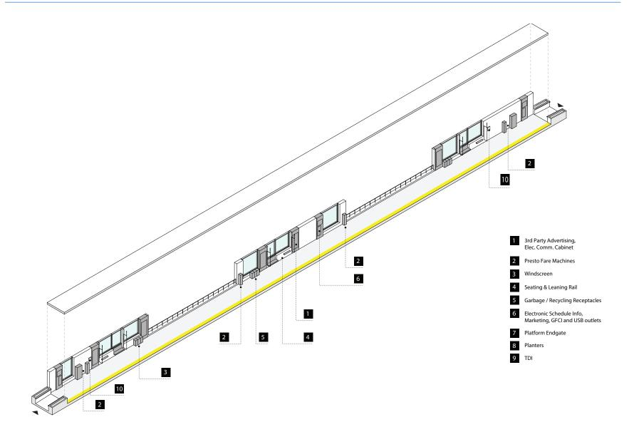
Figure 5-18: Open Shelter at Curbside, Side Platform
