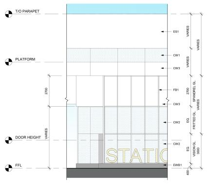
Figure 6-16: Elevation - Station
