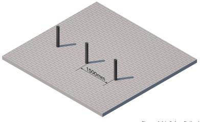
Figure 4-16: Safety Bollards
