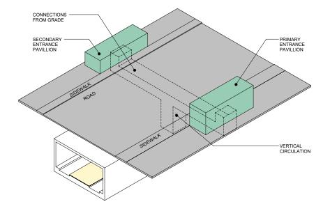
Figure 6-4: Below-grade covered LRT Station - platform under street
