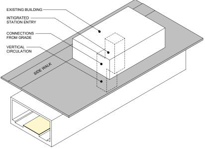
Figure 6-5: Below grade covered LRT station, standalone entrance (left) and integrated entrance in existing building (right)
