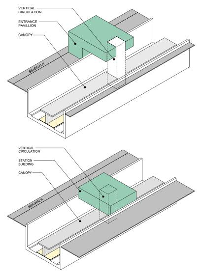
Figure 6-6: Below grade uncovered LRT Station
