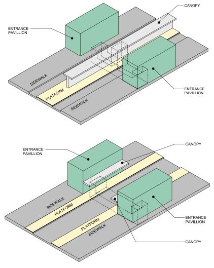
Figure 6-11: At-grade Station - side platform
