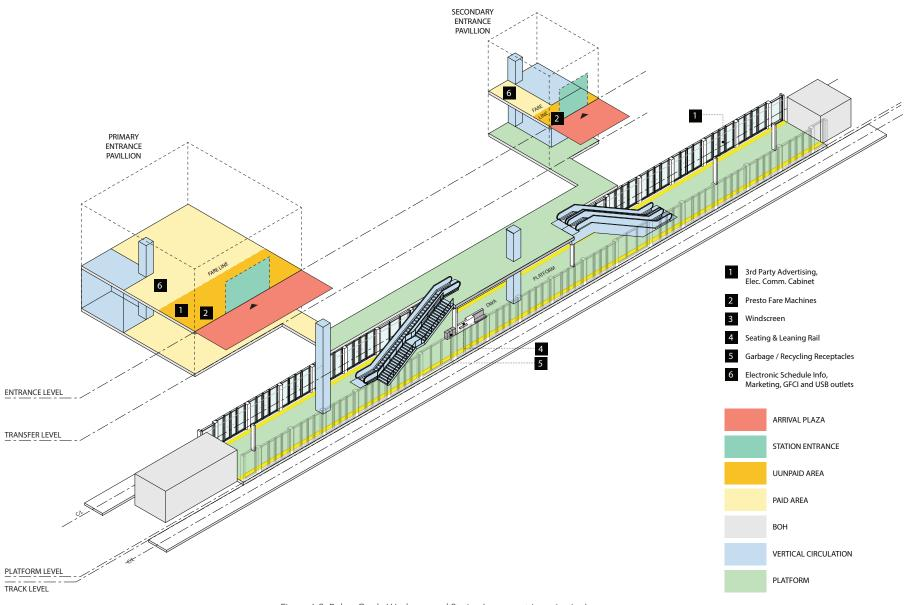
Figure 6-2: Below Grade/ Underground Station (axonometric projection)
